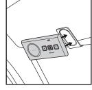
2. Attach the magnet back of the handsfree to the fixed metal clip.
