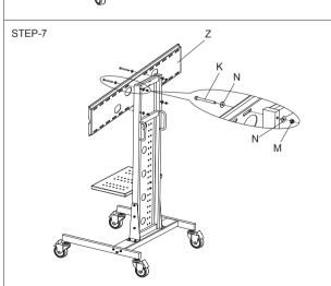
Join the connective plate and supporting pole with M6×65 inner hex bolt pre-through a flat washer and then screw down the bolt with S=5 spanner. Shown as the fig.
