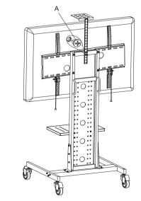
Mount the upper vertical pole assembled with the top plate with four M5×8 bolts as a height needed for the TV and screw down with a cross screwdriver.
