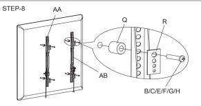
Install the monitor brackets onto the back of the panel TV: screw two bolts into the holes in the back of the panel TV to install each monitor bracket.
