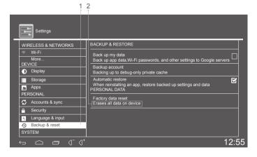
Press Factory data reset under Settings page to (1) to popup the corresponding dialog box. After this selection is confirmed, all the installed software will be erased, once clicking on Erases all data on device (2) and all the settings will reset to the settings the first time the TV turned on.
